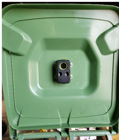
Figure 6: Image of Superfy sensor installed on the lids of 240L carts.
