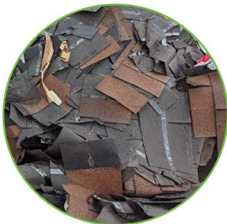
Asphalt roofing shingles can be a valuable recycling resource because of their quantity in CRD waste, ease of separation from other wastes, and the existence of recycling technology and markets. Their use in producing asphalt pavement offers cost savings and may improve roadway performance (Booz Allen Hamilton, 2013). Recycled asphalt shingles can also be repurposed for new shingles or used as a fuel source (Guy Perry and Associates and Kelleher Environmental, 2015).
